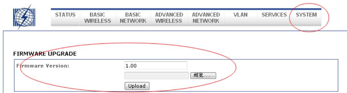
The screenshot shows the 'FIRMWARE UPGRADE' section in the 'SYSTEM' menu. The 'Firmware Version' field is set to '1.00'. Below it is a file upload area with a '浏览...' button and an 'Upload' button.
