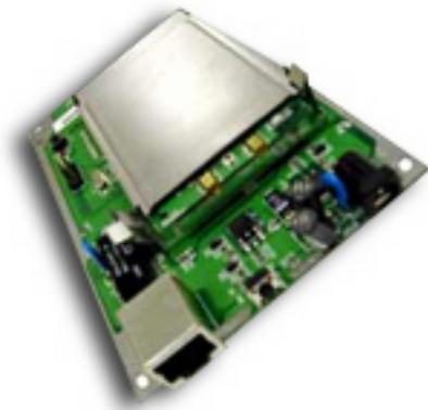
The EZBridge PCB card aims at providing assistance in building a connection between your wired LAN and one or more Wireless Local Area Networks.
