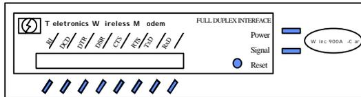
**Fig 4-3. WINC 900A Front Panel**
